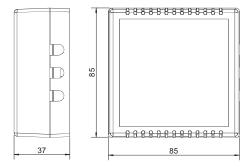
Detach the base of the enclosure by gently pulling along four guiding pins. Fix the base on the wall with two screws. Connect power supply, relay and output cables to the terminal blocks on the PCB and push the enclosure to the base.
