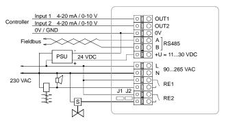
To use analog outputs, connect the terminals OUT1 and/or OUT2 and 0 V to the input of the secondary instrument (indicator or controller). NB! The outputs are not galvanically isolated from 24 V power supply and share common 0 V. Allowed load resistance limits are stated in Specifications table.
